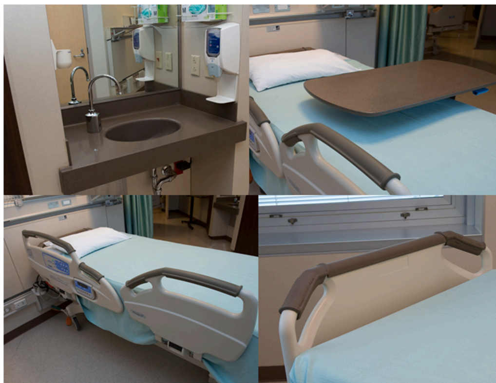
Fig. 1. Copper-oxide infused polymer-based material surfaces installed on sinks, tray tables, and bedrails in patient rooms.
